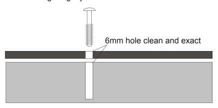
30mm sprint plug hammer in but leave slightly loose.
